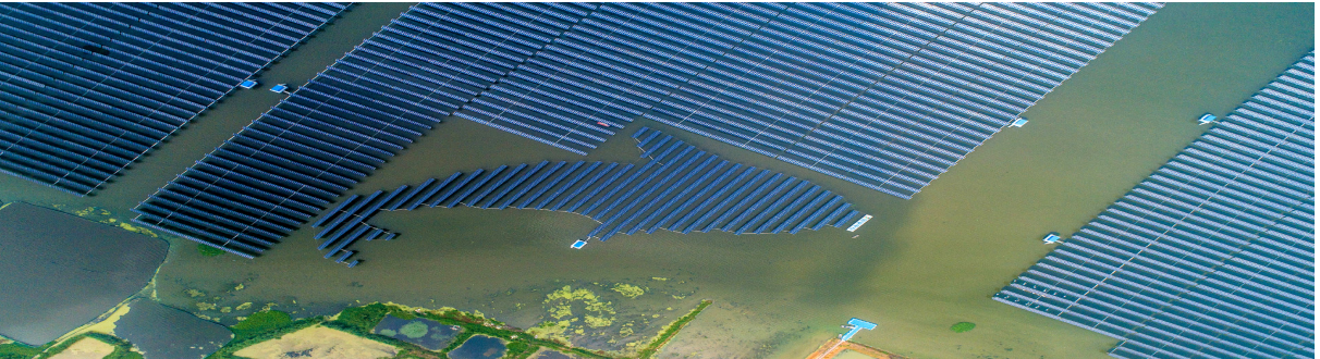
泗洪光伏领跑者基地两期总装机规模1GW，年发电量可达13亿千瓦时，采用农(渔)光互补模式 The total installed capacity of the two phases of Sihong PV Frontrunner Base is 1 GW, with an annual power generation of 1.3 TWh. This project employs agricultural (fishery)- solar complementary mode.
