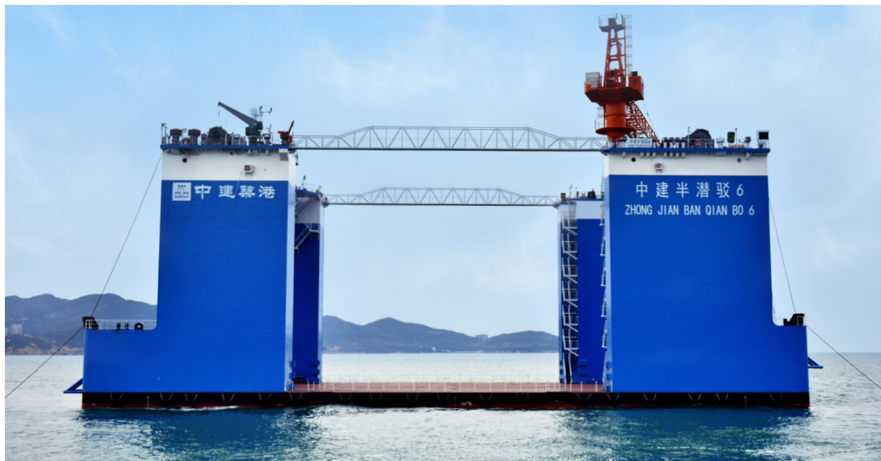
中建半潜驳6 (8000吨级) No.6 Semi-Submersible Barge
