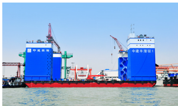
中建半潜驳1 (6000吨级) No.1 Semi-Submersible Barge
