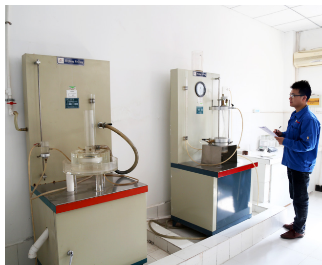
土工织物垂直渗透系数试验 Geotextile Vertical Permeability Coefficient Test
